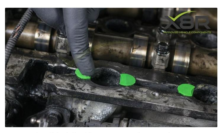
Volvo Swirl Flap Blanking Kit for 2.4L D5 D5244T4 Engines P2015 Fault: Page 18
